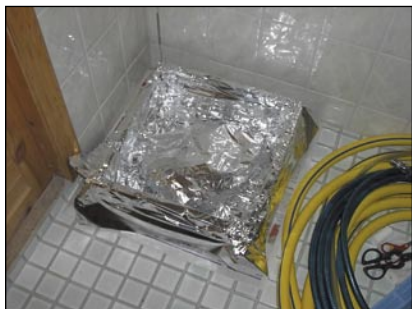
The stone and the glue mold are carefully covered with aluminum foil.
