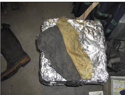
Remove the mould from the artificial stone: start with the edges and peel back gently.
