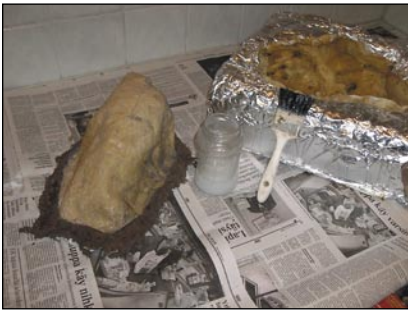
Cover the mould with peeling agent.
