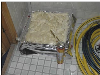
Spray the foam on the foil-covered mould.
