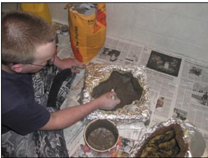
Stroke an even layer of plaster all over the mould and let it dry 24 hours.
